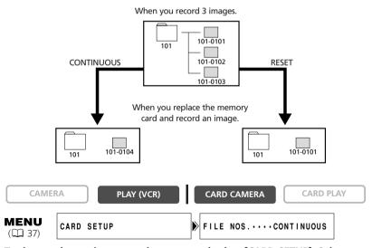
To change the setting, open the menu and select [CARD SETUP]. Select [FILE NOS.], set it to [RESET] and close the menu.
